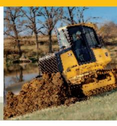
The 700J steers the same and maintains its preset speed whether it's on level ground or a 2-to-1 slope. For total control regardless of the terrain.
