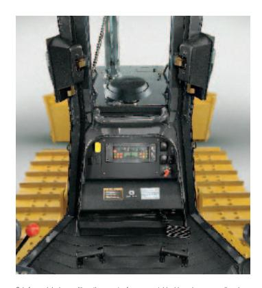
Cab-forward design positions the operator for a more stable ride and a commanding view behind, below, and beyond the blade. Monitor keeps a vigilant watch on vital functions and issues visual or audible warnings.
