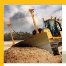
Equipped with optional Intergrated Grade Control (IGC) package, your dozer arrives from the factory "plug and play" ready.
