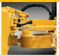
Closed-cell blade design and robot-welded, fabricated, box-section C-frame deliver exceptional strength and durability. Heavy-duty, hardened ball-and-socket joint resists material build-up for long-term grading precision.
