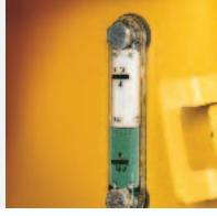
Sight gauges are conveniently located and easy to read for quick hydraulic fluid-level checks.
