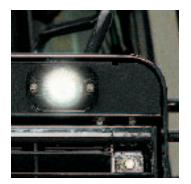
High-intensity halogen driving lights are standard. Or opt for the factoryinstalled 360-degree light package that delivers superior illumination for night work. Turbocharged Deere sixcylinder diesel delivers 86 kW (115 hp) at a low 2,100 rpm, for good fuel economy, longevity, and reduced noise. One-piece robot-welded mainframe resists torsional stress, absorbs shock loads, and delivers maximum strength while providing easy service access to major drivetrain components.
