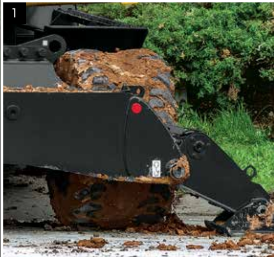
1. Heavy-duty covers on the oversize outriggers help prevent damage to the hydraulic cylinders.
