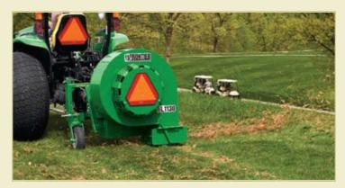
The BL1130 provides 141 miles-per-hour of maximum air velocity and 6,000 cubic feet-per-minute of maximum airflow so you can blow through chores with ease.
