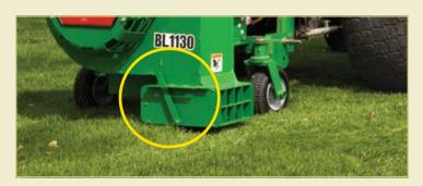
Use this handy adjusting lever (highlighted) to change leftright position of the discharge outlet.
