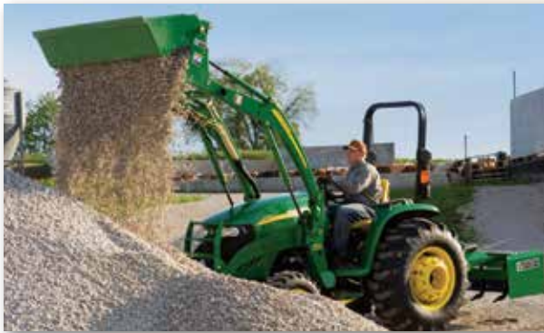
The 4-in-1 Bucket makes moving loose material fast and easy. Simply scoop the material up and haul it. The bucket clam seals shut, keeping material locked in. And with the high-dump capability (above), you can deposit material right where you want it, even in trenches and dump trucks. You also can meter the material as the bucket jaws are opened.
